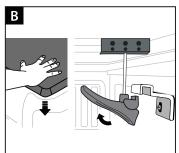
B: WITH ONE HAND, LIFT AND KEEP THE LATCH HANDLE POINTING UP AS MUCH AS POSSIBLE (BEYOND 90°). THEN, WITH THE OTHER HAND FIRMLY PRESSED DOWN ONTO THE COVER CORNER. CONTINUE TO ROTATE HANDLE TO ADJUST THE POSITION.
