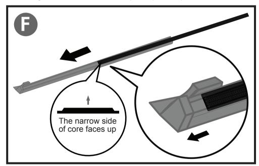
Insert sealed/stitched end of new velcro into the aluminum rail channel.
