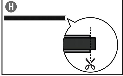
Use Adhesive Adjustment Strip to pull velcro strip all the way to the end of channel.
