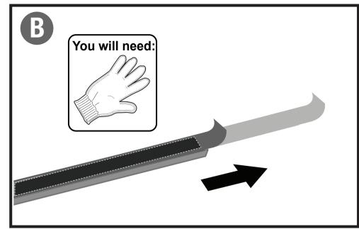
With gloves on, use Adhesive Adjustment Strip to pull to-be replaced (old) velcro strip out of the aluminum channel.
