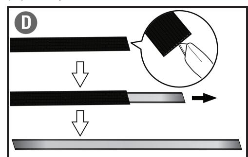
Cut along the end of old velcro strip and pull out plastic core.
