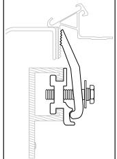
FOR NISSAN TITAN WITH FACTORY UTILITY TRACK, REFER TO THE ILLUSTRATION TO THE LEFT ON HOW TO SLIDE THE BRACKETS INTO THE TRACK AND TO HELP VISUALIZE THE CORRECT WAY TO TIGHTEN THEM.
