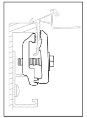
• FOR NISSAN FRONTIER WITH FACTORY UTILITY TRACK, REFER TO THE ILLUSTRATION TO THE LEFT ON HOW TO SLIDE THE BRACKETS INTO THE TRACK AND TO HELP VISUALIZE THE CORRECT WAY TO TIGHTEN THEM. REFER TO THE ILLUSTRATION IN PAGE 2 TO DETERMINE TO THE CORRECT BRACKET POSITIONING.
