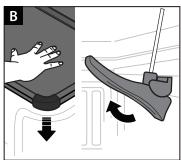
B: WITH ONE HAND, LIFT AND KEEP THE LATCH HANDLE POINTING UP AS MUCH AS POSSIBLE (BEYOND 90°). THEN, WITH THE OTHER HAND FIRMLY PRESSED DOWN ONTO THE COVER CORNER. CONTINUE TO ROTATE HANDLE TO ADJUST THE POSITION.
