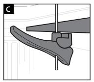
C: FOR THE TIGHTEST FIT, OPENING OF LATCH JAW SHOULD BE LEVEL WITH THE SIDE RAIL LIP WITHOUT LIMITING ACCESS TO THE JAW.
