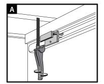
A: Start by pulling down latch handle from the back of cover. Then unscrew the handle to lower its position.
