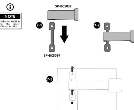
• Turn the knob counterclockwise to loosen the safety clamp with the strap, attach clamp to the metal bed rail lip on both sides, then tighten.
