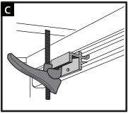
${\bf C:}$  For the tightest fit, opening of latch jaw should be level with the side rail lip without limiting access to the jaw.
