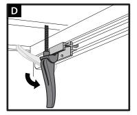
**D:** Latch the jaw groove fully into the rail lip, then crank handle down to tighten. Go back and readjust jaw position from step b if the latch does not feel very tight.
