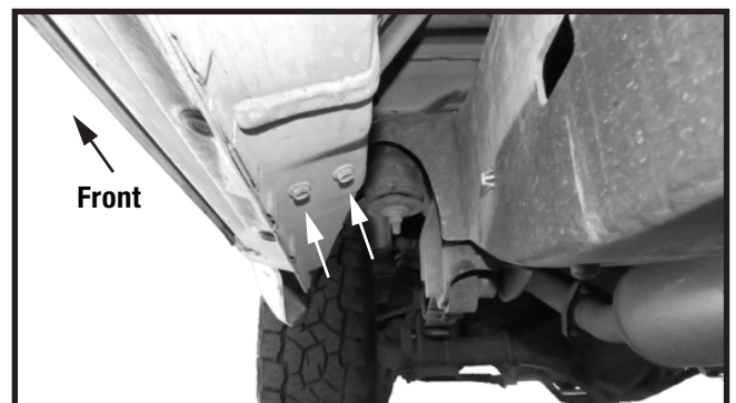
(Fig 10) Locate Passenger/Right side rear mounting location. Attach Passenger/Left 3rd/Rear Mounting Bracket [F] to mounting location using same hardware as Fig 2. Remove any plastic plugs or bolts in the threaded inserts
