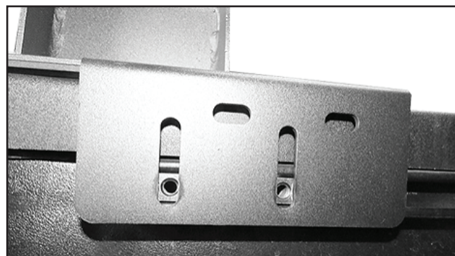
(Fig 14) With assistance, place the Overland Bed Rack assembly onto the top of the bed. Line up the Block Nuts to the desired slots, (2) Block Nuts per mounting plate
