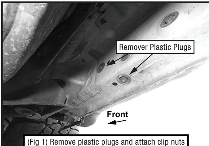
(Fig 1) Remove plastic plugs and attach clip nuts to **front** mounting location
