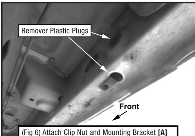
(Fig 6) Attach Clip Nut and Mounting Bracket [A] to 2nd center mounting location (Refer to Fig 2-3)
