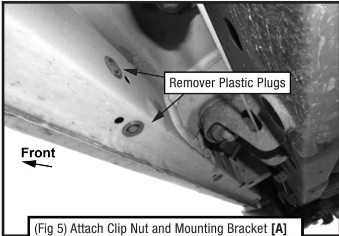
(Fig 5) Attach Clip Nut and Mounting Bracket [A] to 1st center mounting location (Refer to Fig 2-3)
