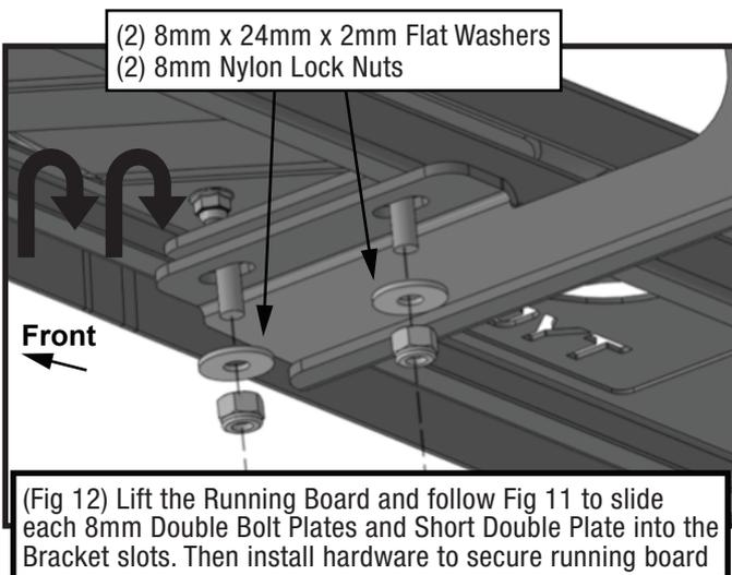
(Fig 12) Lift the Running Board and follow Fig 11 to slide each 8mm Double Bolt Plates and Short Double Plate into the Bracket slots. Then install hardware to secure running board
