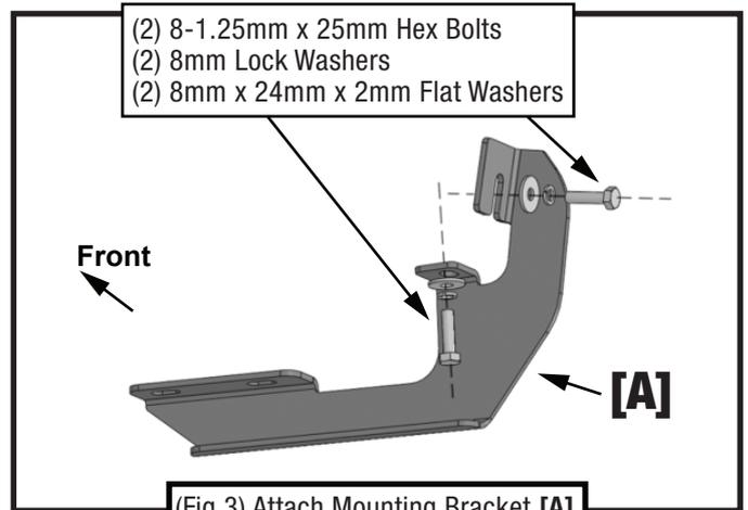
(Fig 3) Attach Mounting Bracket [A]
