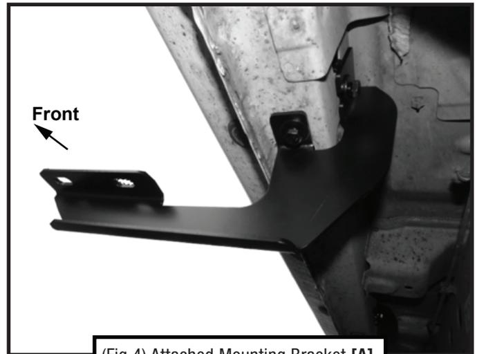
(Fig 4) Attached Mounting Bracket [A]
