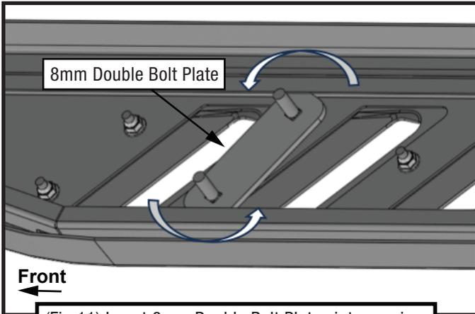
(Fig 11) Insert 8mm Double Bolt Plates into running board channels for Mounting Brackets [A]
