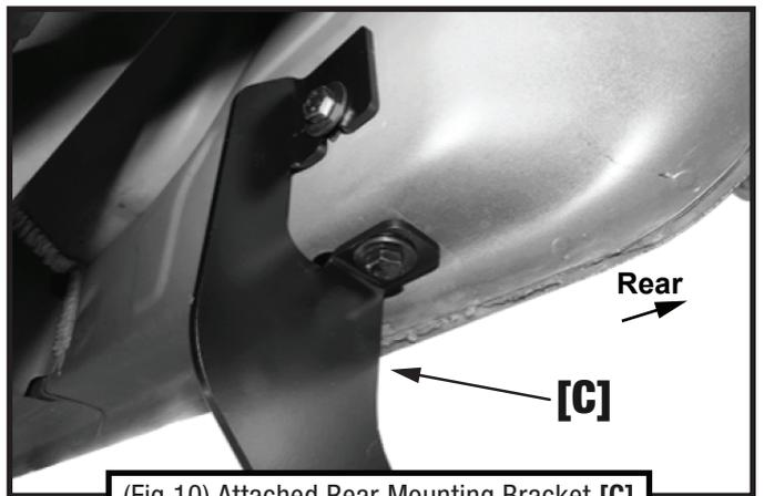
(Fig 10) Attached Rear Mounting Bracket [C]
