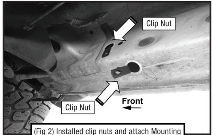
(Fig 2) Installed clip nuts and attach Mounting Bracket [A] to **front** mounting location
