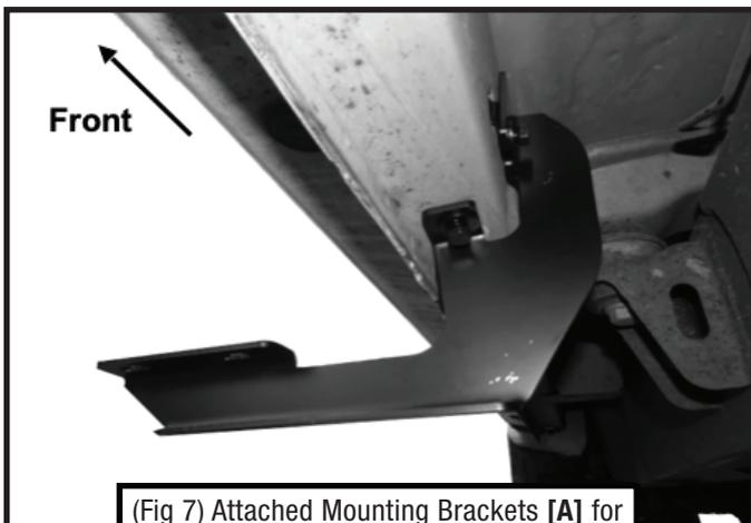
(Fig 7) Attached Mounting Brackets [A] for 1st and 2nd center mounting locations
