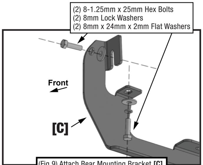
(Fig 9) Attach Rear Mounting Bracket [C]
