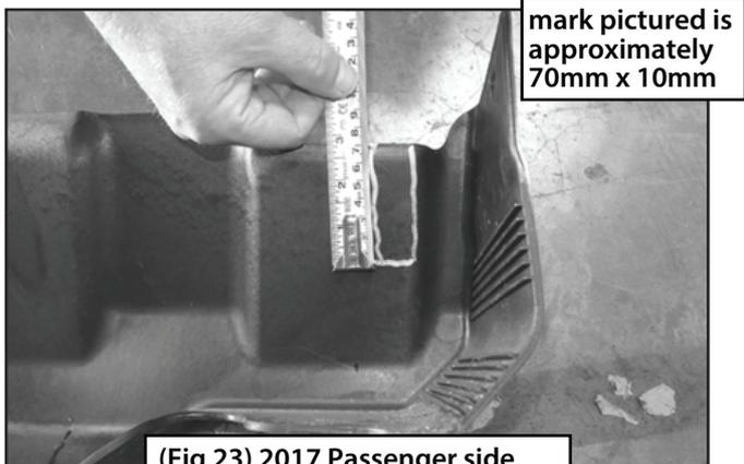
(Fig 23) 2017 Passenger side DEF cover marked for trimming
