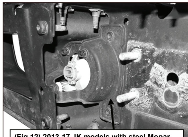
(Fig 12) 2013-17 JK models with steel Mopar option bumper and 2-tab, 3-post halogen fog light assembly, remove assembly from bumper (passenger/right side pictured)
