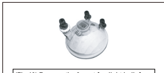
(Fig 13) Remove the 3-post fog light bulb from the plastic bracket assembly (see Fig 12)
