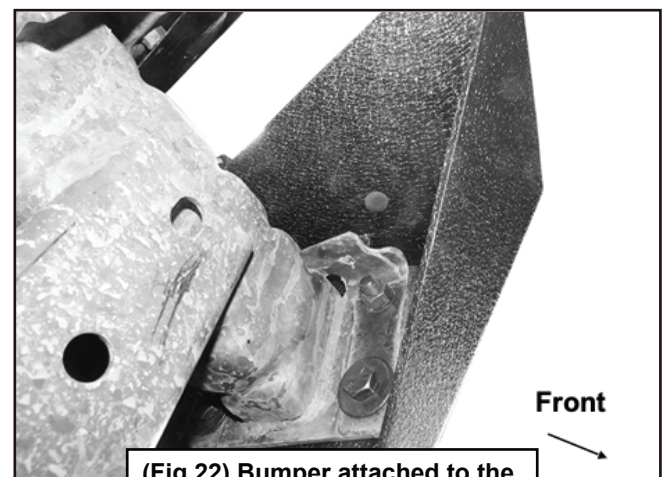
(Fig 22) Bumper attached to the passenger/right mounting plate
