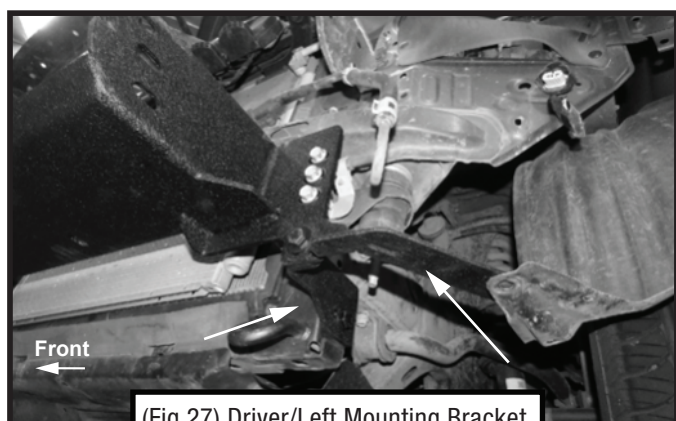
(Fig 27) Driver/Left Mounting Bracket and Support Bracket installed
