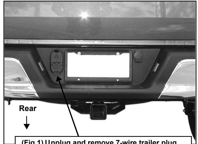
(Fig 1) Unplug and remove 7-wire trailer plug
