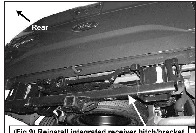
(Fig 9) Reinstall integrated receiver hitch/bracket assembly on models with "HD Towing" package
