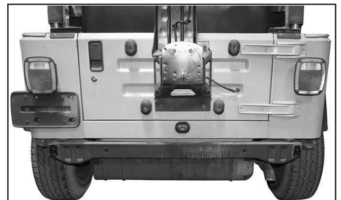
(Fig 2) Remove bumper bolt from the bottom of the frame (arrow). Remove hex nuts attaching bumper to frame (passenger/right side pictured)
