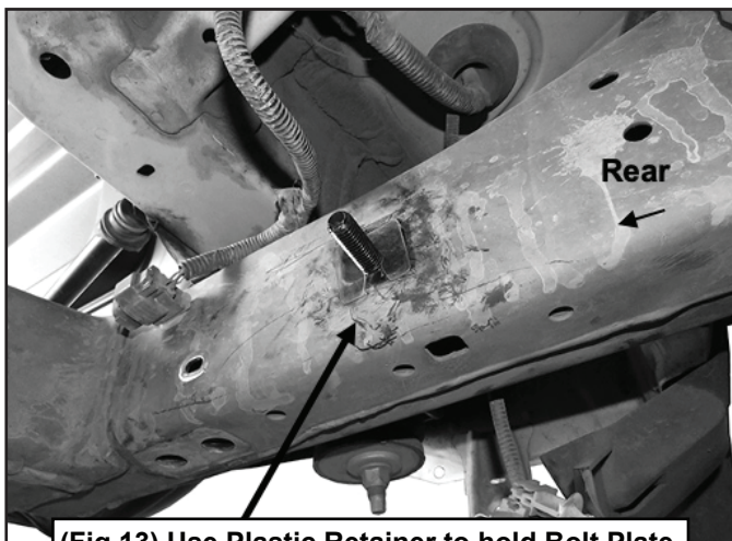
(Fig 13) Use Plastic Retainer to hold Bolt Plate
