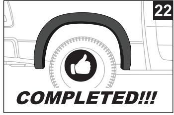
22. Tightly press flare against vehicle to evenly remove space between flare and vehicle. Tighten all 10 screws. Installation complete.
