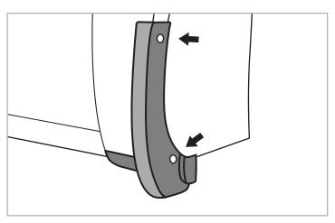
**STEP 2:** Remove 2 factory screws and the mudflap with 8mm socket. Hold onto the screws to be reused in STEP 4.
