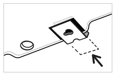
**STEP 9:** Stick a supplied Tab **[F]** over the factory hole and slide a supplied U-clip **[G]** over the Tab as shown.
