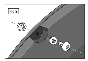
**IMPORTANT:** Do not drill holes to the vehicle body as rivets are decorative and fasten only to the flare. Do not attempt to use the bolts to fasten flare to vehicle body.
