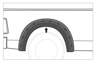
**STEP 11:** Position flare to vehicle. Install a supplied PH Truss Screw **[H]** through the flare and into the U-clip. Do not tighten.
