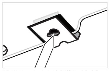
STEP 10: With an awl, poke a hole in the Tab through the U-clip.
