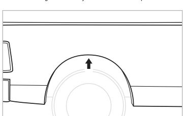
**STEP 8:** Locate top factory screw hole position.
