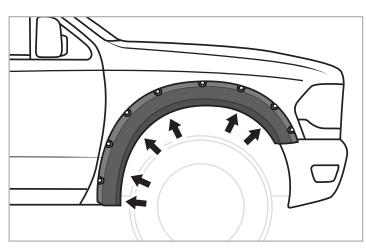
**STEP 4:** Hold flare into position and reinstall 6 factory screws kept from STEPs 2-3 with 8mm socket. Do not tighten.
