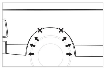
**STEP 7:** Uninstall 6 factory screws with 8mm socket from the pointed positions. (Keep the X location screws installed) Hold onto screws to be reinstalled in STEP 12.
