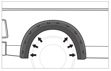
**STEP 12:** Reinstall 6 factory screws from STEP 7 to the same 6 positions with 8mm socket. Do not tighten.
