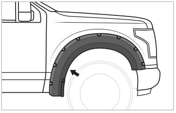
**STEP 9:** With a PH Screwdriver, install a PH Truss Screw [I] through hole in flare and into clips installed in Step 3.
