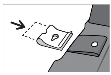
**STEP 4:** Slide 3 supplied U-clips **[H]** onto the right inner bracket. NOTE: Right Inner Bracket has 'RR' marked on it.
