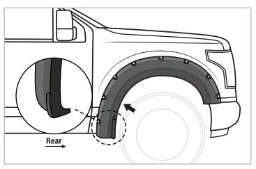
**STEP 2:** With a grease pencil, mark 1 locations as indicated using hole in flare as guide.
