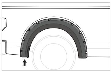
**STEP 18:** Install a supplied Plastic Retainer [M] into hole in flare and vehicle's factory hole.
