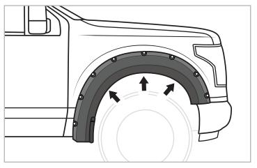
**STEP 7:** Hold flare in position, install 3 supplied PH Truss Screws [I] through holes in flare and into holes in clips on the inner piece installed in Step 4. Do not tighten.
