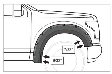
**STEP 8:** With the incidated tools above, reinstall the factory screws removed in Step 1.
