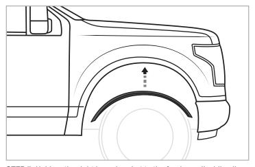
**STEP 5:** Hold up the right inner bracket to the fender well while aligning the 3 holes in the bracket with vehicle's top 3 factory holes.
