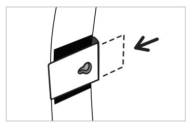
**STEP 3:** Stick a supplied Tab **[F]** over the mark made in Step 2, and wrap the Tab around the metal lip. Then, slide a Long U-clip **[G]** over the Tab.
