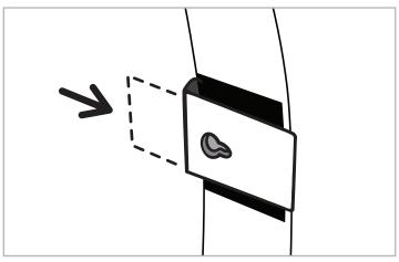
**STEP 12:** Stick the supplied Tabs **[F]** over the 4 mark locations indicated in Step 13, and wrap the Tabs around the metal lip. Then, slide a Long U-clip **[G]** over each Tab.
