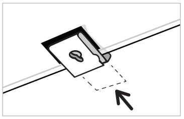
**STEP 14:** Stick a supplied Mylar Tab **[J]** over the last remaining mark indicated in Step 15. Then slide a supplied S-clip **[K]** over the Mylar Tab.
