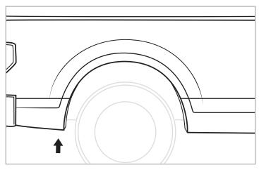
STEP 10: Remove factory screw from bottom rear of fender well.
