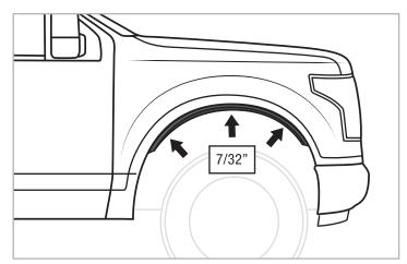
**STEP 6:** With a 7/32" socket wrench, reinstall 3 factory screws to secure the inner piece to the fender well.
