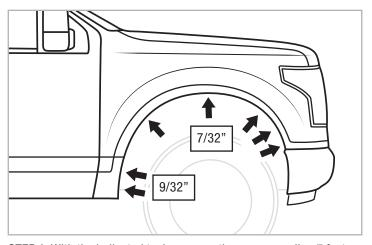
**STEP 1:** With the indicated tools, remove the cooresponding 7 factory screws and keep for later use.
