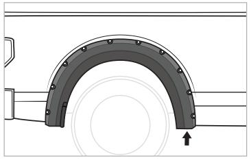
**STEP 17:** Install a supplied PH Metal Screw **[L]** through hole in flare and into S-clips installed in Step 14.
