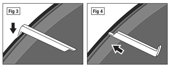
**STEP 19:** If needed use supplied tool **[N]** to trim outer edge (Fig 3) and inner edge (Fig 4) by inserting tool ends then sliding around the entire edge trims from one end to the other as shown in above pictures.
