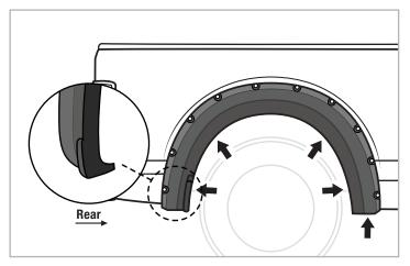
**STEP 11:** Hold flare in position. With a grease pencil, mark 5 locations using holes in flare as guide. Then, remove flare.
