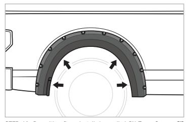
**STEP 16:** Reposition flare, install 4 supplied PH Truss Screws **[I]** through holes in flare and into the Long U-clips installed in Step 12.
