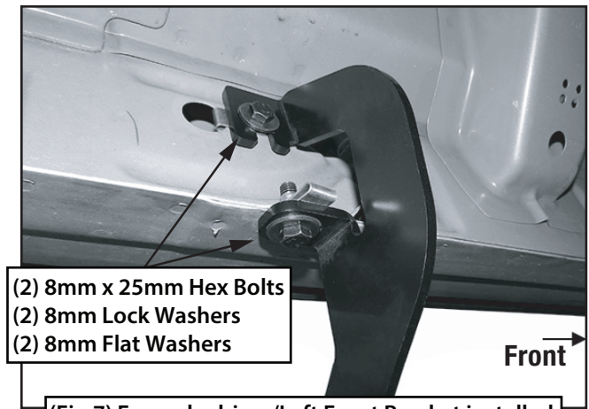
(Fig 7) Example driver/Left Front Bracket installed.
