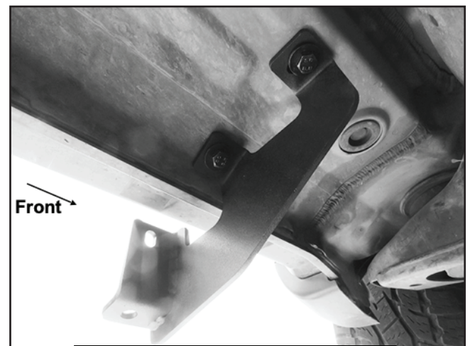
(Fig 5) Driver/Left Front Mounting Bracket attached to the front location
