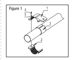
Slide the Lower Clamp Mount into the slot in the Upper Clamp Mount. Wrap the Upper and Lower Clamp Mount around the plastic ring, (Figure 1).
