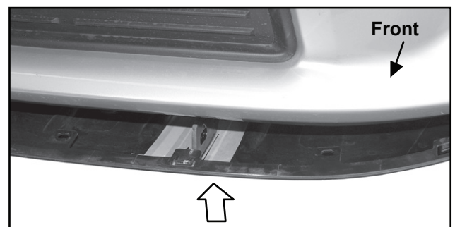
(Fig 15) Hold the splash guard up to the bottom of the brackets and mark location for cutting to clear brackets. Cut only what is needed to insert bracket through the splash guard.
