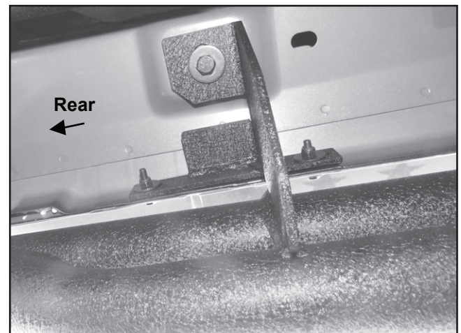
(Fig 6) Driver/left side rear welded Bracket installed
