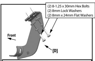
(Fig 11) Attaching Passenger/Right Center/Rear Mounting Bracket [**D**] to Passenger/Right rear mounting location with indicated hardware
