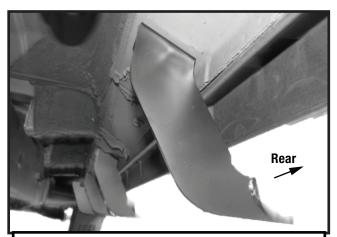
(Fig 12) Attached Passenger/Right Center/Rear Mounting Bracket [**D**] to Passenger/Right rear mounting location
