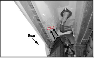
(Fig 10) Locate Passenger/Right side <u>rear</u> mounting location. Attach Passenger/Right Center/Rear Mounting Bracket [**D**] to mounting location using same hardware as **Fig 2**. Remove any plastic plugs in the threaded inserts
