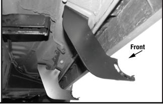
(Fig 9) Attached Passenger/Right Center/Rear Mounting Bracket [**D**] to Passenger/Right 2nd center mounting location
