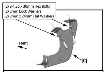
(Fig 2) Attach Passenger/Right Front Mounting Bracket **[C]** to Passenger/Right Front mounting location with indicated hardware
