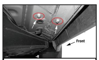
(Fig 1) Locate Passenger/Right side front mounting location. Remove any plastic plugs in the threaded inserts
