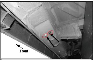
(Fig 7) Locate Passenger/Right side <u>2nd</u> Center mounting location. Using same hardware as **Fig 2**, remove any plastic plugs in the threaded inserts
