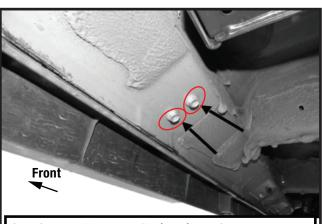
(Fig 4) Locate Passenger/Right side <u>1st</u> Center mounting location. Using same hardware as **Fig 2**, remove any plastic plugs in the threaded inserts
