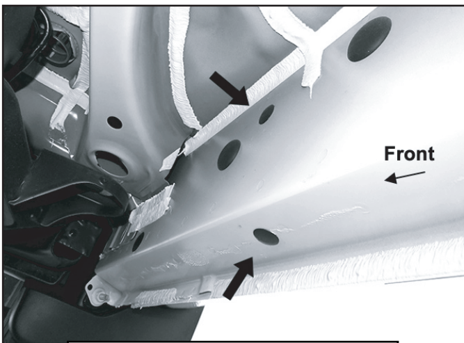
(Fig 1) Remove plastic plugs (arrows) to uncover threaded holes in floor
