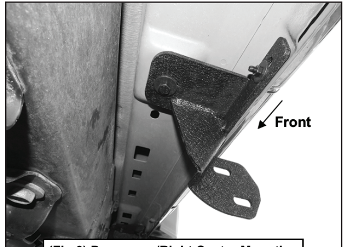
(Fig 6) Passenger/Right Center Mounting Bracket attached to the center location
