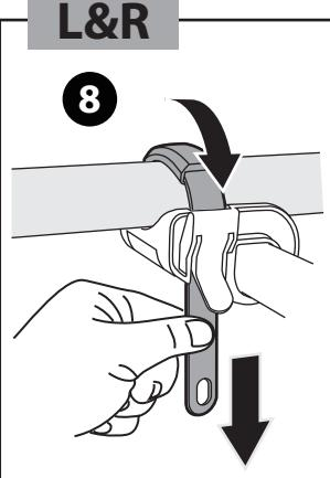
**EN** Must use the included safety straps to attach the bikes to the bike carrier, and to stabilize the bikes & wheels to avoid swinging and scratching during driving.
