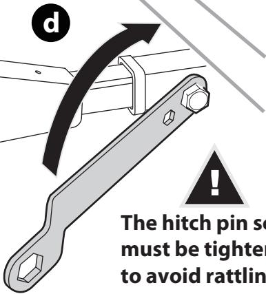
! The hitch pin screw must be tightened to avoid rattling.
