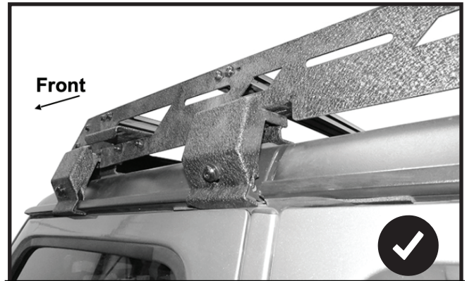
(Fig 14) Front & Second Bracket Clamp Covers installed
