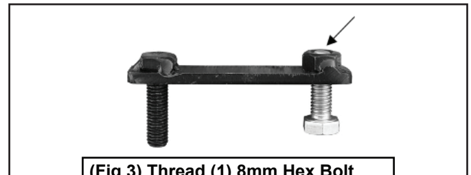
(Fig 3) Thread (1) 8mm Hex Bolt into the nut on the plate. Stop when bolt reaches end of nut as pictured
