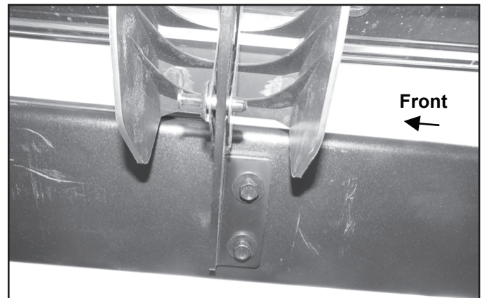
(Fig 12) Passenger/right Sidebar attached to Mounting Bracket at the center location
