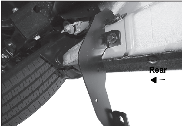
(Fig 11) Driver/Left Rear Mounting Bracket installed
