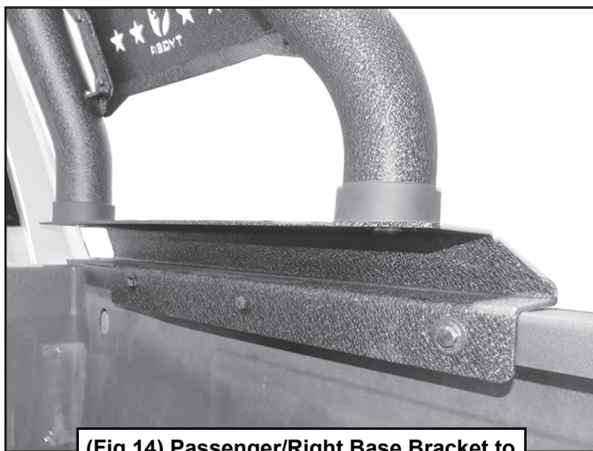
(Fig 14) Passenger/Right Base Bracket to bed installed
