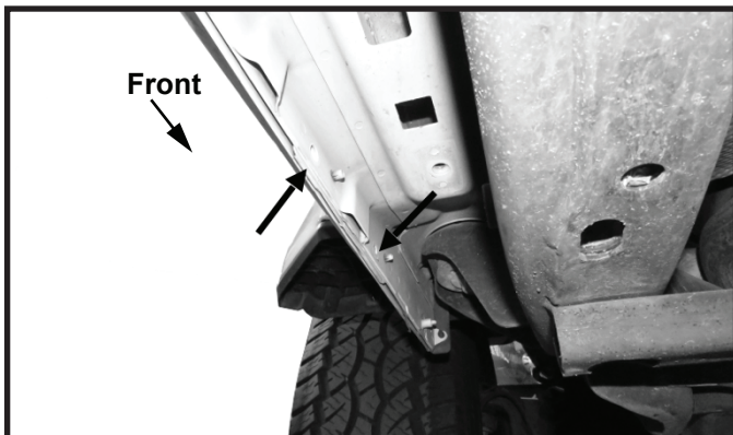
(Fig 1) Starting at Driver Side Front, locate the mounting points and attach Driver Side Front Support Bracket [I] to pinch weld
