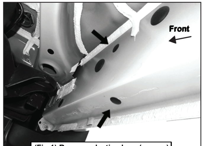
(Fig 1) Remove plastic plugs (arrows) to uncover threaded holes in floor
