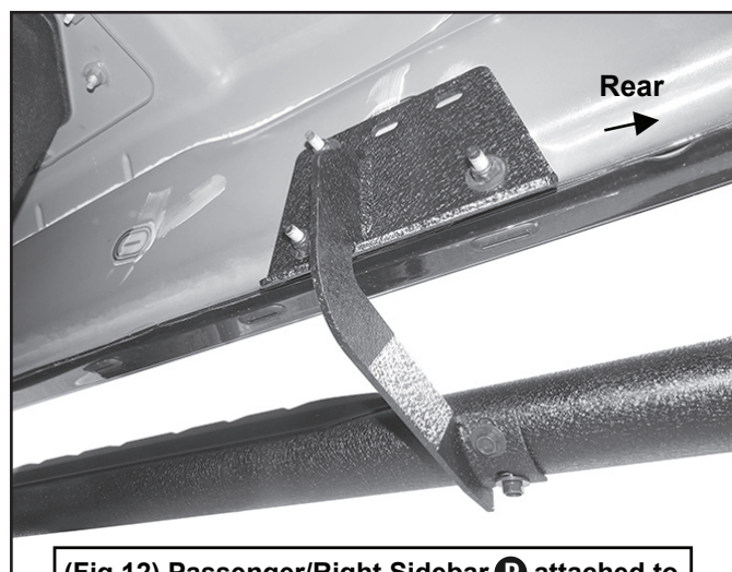
(Fig 12) Passenger/Right Sidebar P attached to rear Bracket
