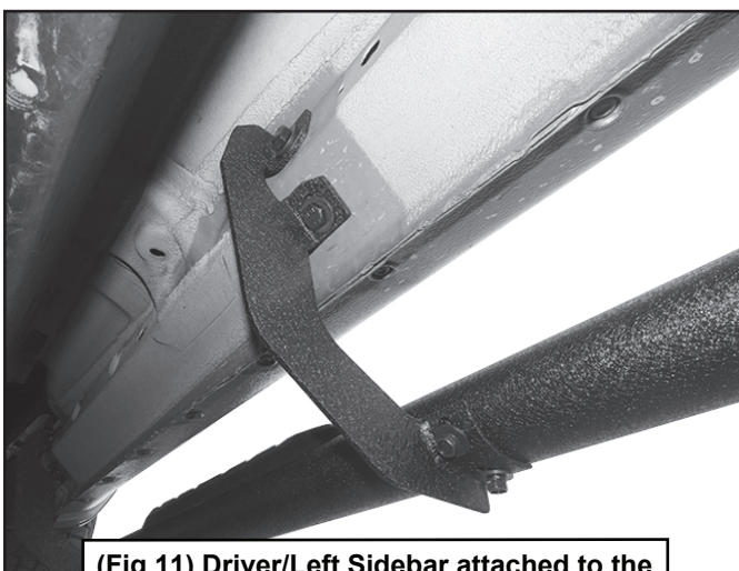
(Fig 11) Driver/Left Sidebar attached to the Center Mounting Bracket
