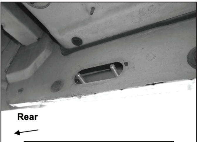
(Fig 5) 4-door Driver/Left Rear Mounting location. Insert large Double Bolt Plate
