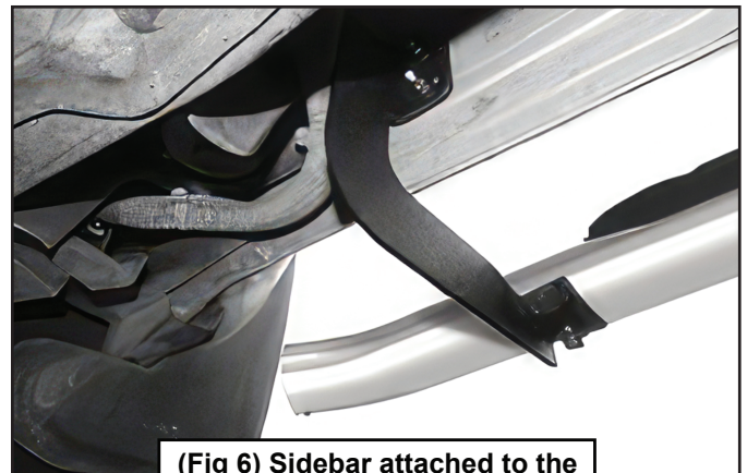
(Fig 6) Sidebar attached to the Front Mounting Bracket
