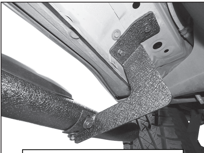
(Fig 11) Driver/Left Sidebar attached to the Front Mounting Bracket
