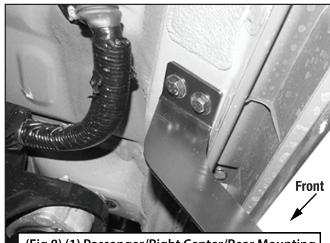
(Fig 8) (1) Passenger/Right Center/Rear Mounting Bracket [D] attached to the rear location
