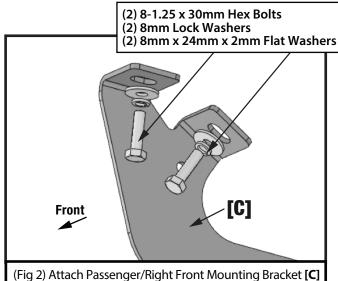
(Fig 2) Attach Passenger/Right Front Mounting Bracket **[C]** using indicated hardware to the <u>front</u> mounting location. DO NOT fully tighten hardware at this time
