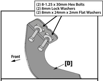
(Fig 5) Attach Passenger/Right Center Mounting Bracket [D] using indicated hardware to the <u>center</u> mounting location. DO NOT fully tighten hardware at this time
